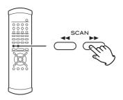
When playing back, use the SCAN button (◀◀ or ►►) to move backwards and forwards (sound is muted for DVD video and video CD discs). Press PLAY to restart playback at normal speed at the desired location.
